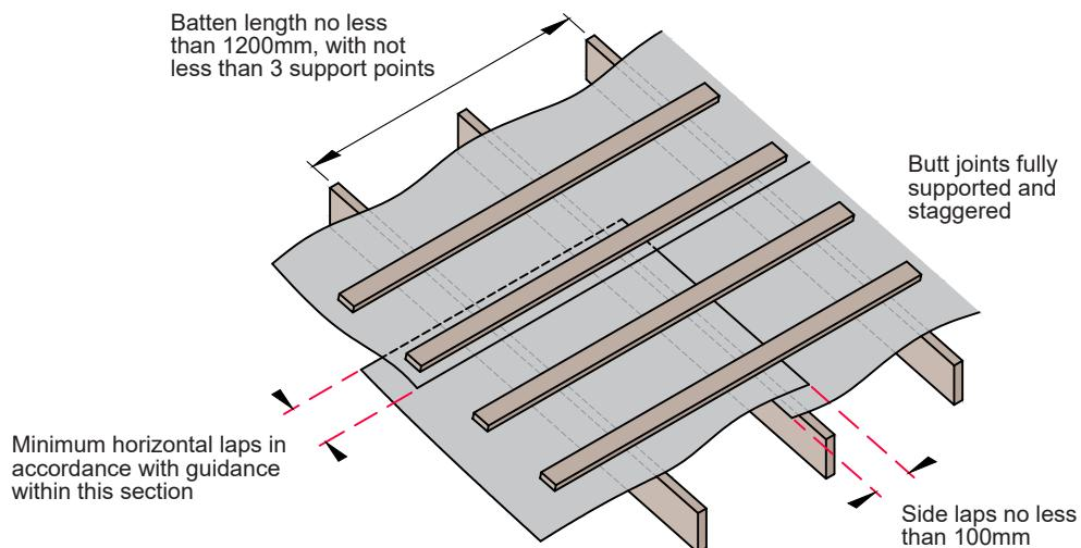
The lap of the underlay should be secured in accordance with the manufacturers third party product conformity certificate.
