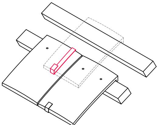
Tile clips may need to be utilized to achieve a subtitle number of fixings to comply with BS 5534 especially on hips or valleys. Tile clips provide resistance to the applied overturning moment more successfully than a nail fixing. The latter is closer to the pivot line, where the nib touches the batten and cannot resist the uplift force at the tail.
