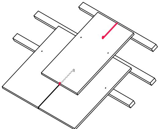
Hooks are formed from stainless steel wire conforming to BS 1554 grade 316 S11 or 316 S19. For further advice on the use of slate hooks, refer to BS 5534 section 4.12.3 and 5.3.6.4 Hooks and rivets for slates. Slates should not be nailed to accommodate hooks.
