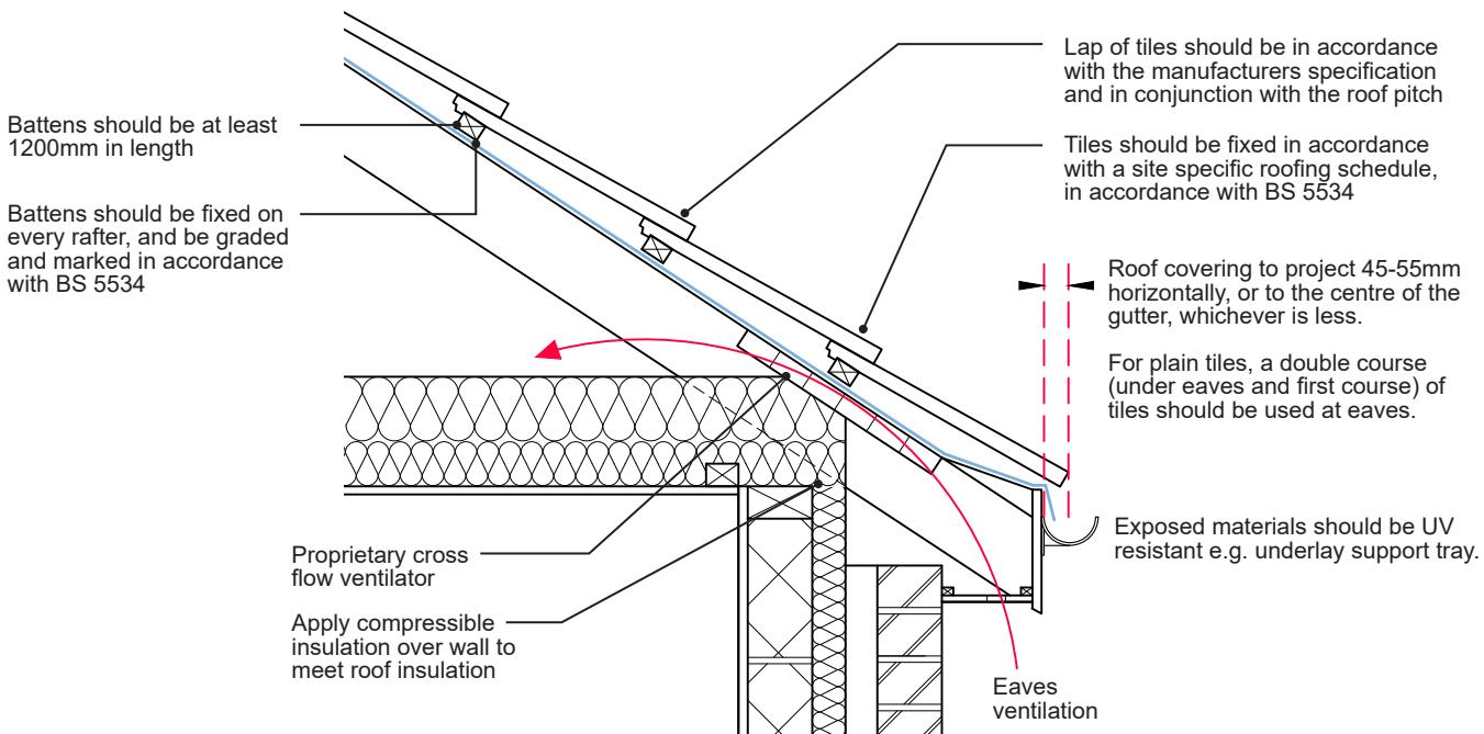
BS 5534 recommends the use of aluminium or stainless steel nails under normal conditions of exposure. Plain or galvanised nails may be used for fixing battens to rafters, but care must be exercised when there is high humidity as certain timber preservative treatments may corrode steel, zinc or aluminium. For all roof areas and rafter pitches, every tile should be mechanically fixed.
